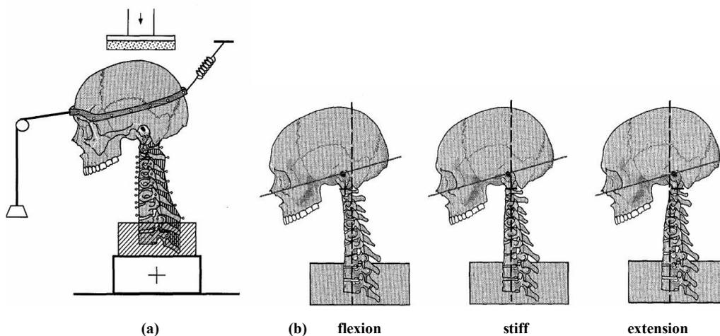
Figure 1. (a) Experimental setup showing the positioning of the cadaver and loading applied
