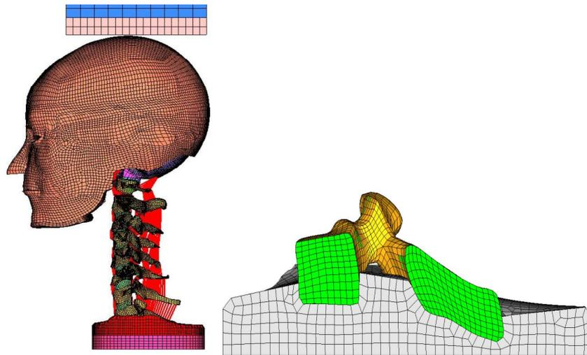
Figure 2. (a) FE model setup (b) T1 fixed to the casting
