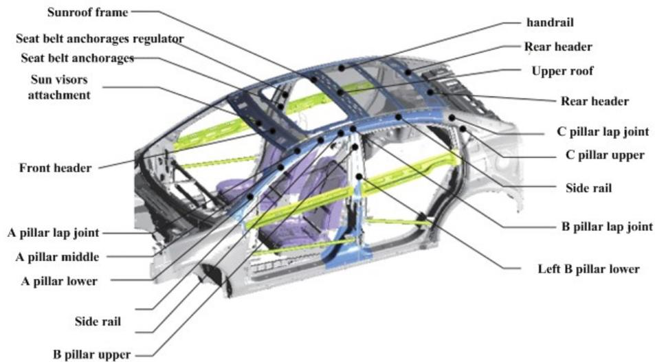
Figure 1. Impact points in vehicle upper part
