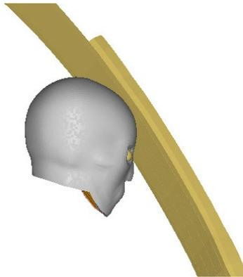
**Figure 5. A-pillar impact simulation**
