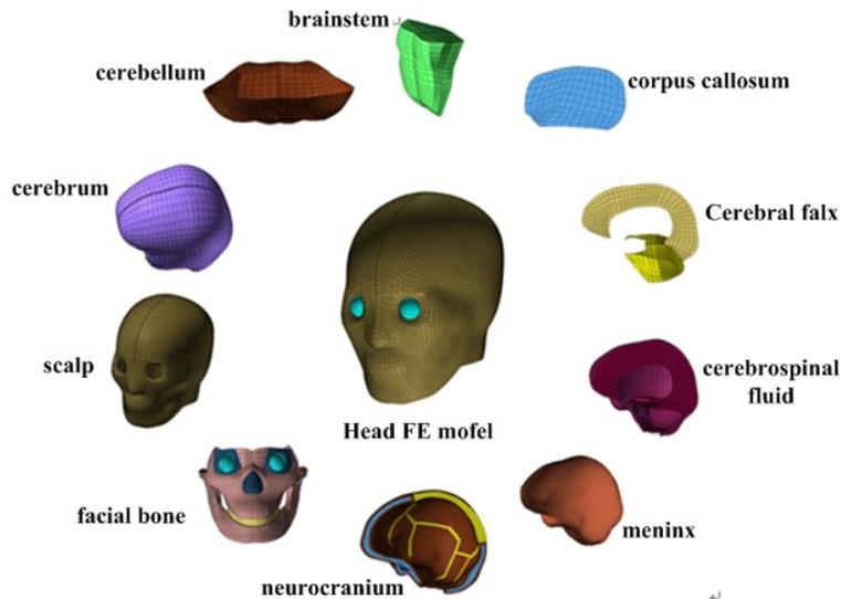
Figure 4. Modified head finite element model
