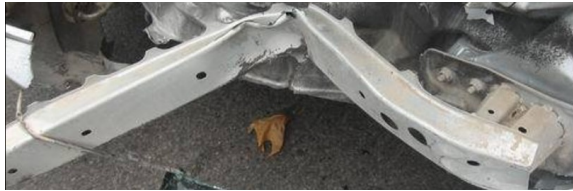
Figure 2 Deformation of a bumper beam after local frontal crash
