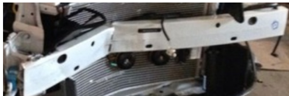
Figure 3 Deformation of a bumper beam after low speed crash
