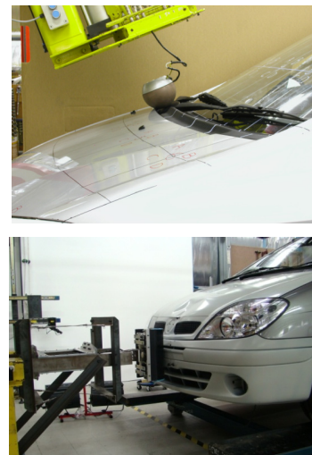
Figure 3. Illustrative example of tests to determine contact-impact properties. The location is that identified in the accident investigation. The speed and angle are determined from the preliminary MADYMO simulation
