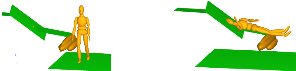
Figure 1. An illustrative example of MADYMO simulation reconstructing one of the pedestrian cases in this study. The top frame is just before the collision and the bottom frame is at head impact
