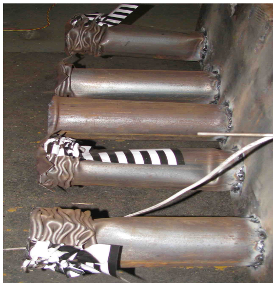
Figure 6. The deformation of circular energy absorption tubes in sled crash test
