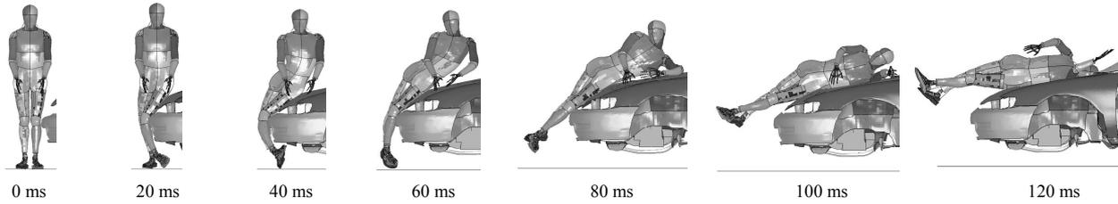
Figure 3. Kinematic behaviour of pedestrian in medium car collision
