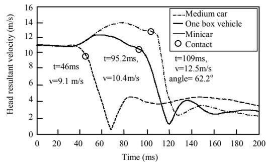
Figure 6. Head resultant velocity relative to vehicle
