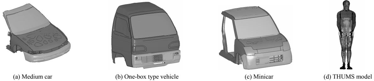
Figure 1. FE models for simulations
