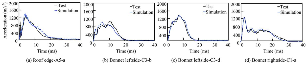
Figure 2. Headform impact test validation
