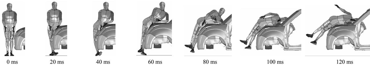
Figure 5. Kinematic behaviour of pedestrian in minicar collision
