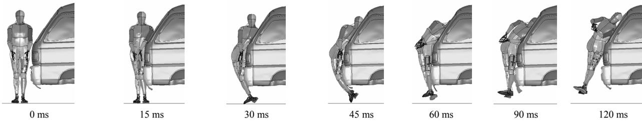
Figure 4. Kinematic behaviour of pedestrian in one box type vehicle collision
