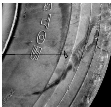
Figure 6. scratched mark of sidewall
