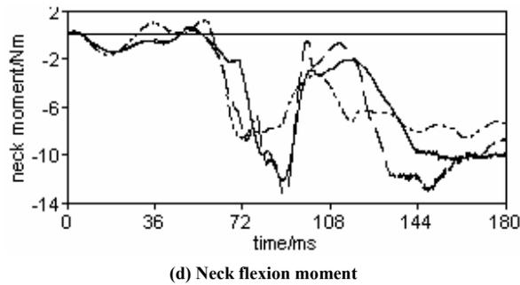
**Figure 7. Injury parameters curves obtained from simulations of CRS without top tether ( ——— Seatbelt without tether — — — LATCH without tether - - - - - ISOFIX without tether)**
