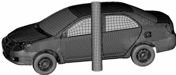
Figure 1. Pole side impact FE model
