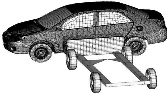
Figure 3. Side impact FE model Figure
