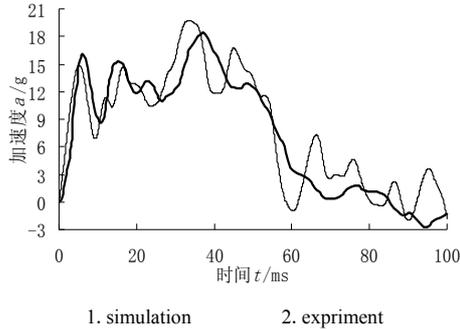
Figure 4. Acceleration curves for simulation and experiment
