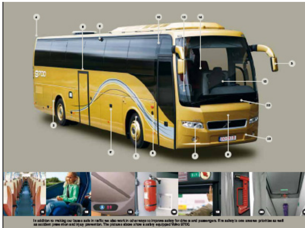
Figure 7. Technologies aimed at improving coach safety (1 Electronic Disc brake & ESP, 3 + 4 «All around» rear view, 19 + 21 Emergency exits, 12 to 16 Restrain systems, 23 Front underrun, 10 Rollover protection, 6 + 7 Improved lighting, 11 + 22 Interior protection, 18 to 21 Passenger evacuation)
