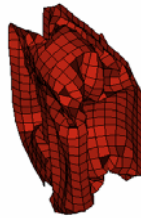
Figure 9 Deformation of crashbox I
