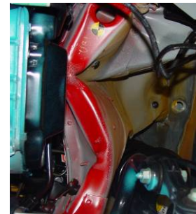
Figure 17 Longeron deformation of test
