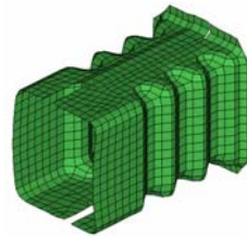
Figure 7 The deformation of the longeron
