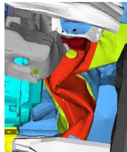
Figure 16 Deformation of longeron
