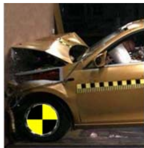
Figure 15 Front deformation of test
