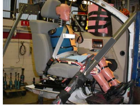
Figure 13: Initial position of Dummy and Seat relative to Door
