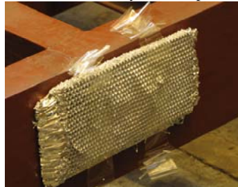
Figure 3: The structure of impact attenuator after crash testing
