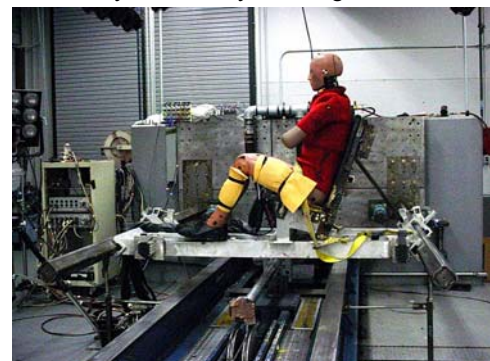
Figure 2: Set-up of the rigid seat with seated dummy
