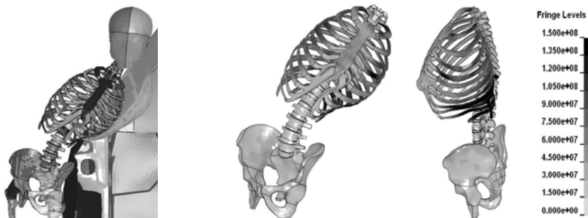
Figure 7 Pedestrian skeleton deformation and von Mises stress distribution in the collision with one-box type vehicle
