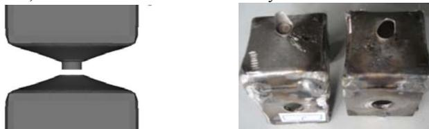
Figure 7. The comparison of failure from computer simulation and tested specimens.
