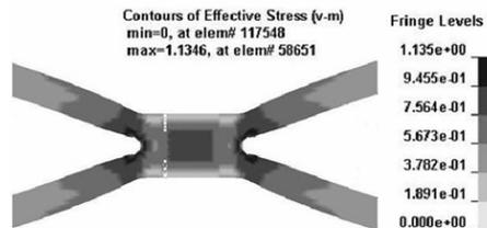
Figure 9. The effective stress contour of spot-weld area at the time of initial fracture
