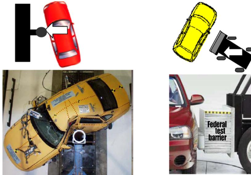
Figure 1 Barrier and pole crash test schematic of New FMVSS214
