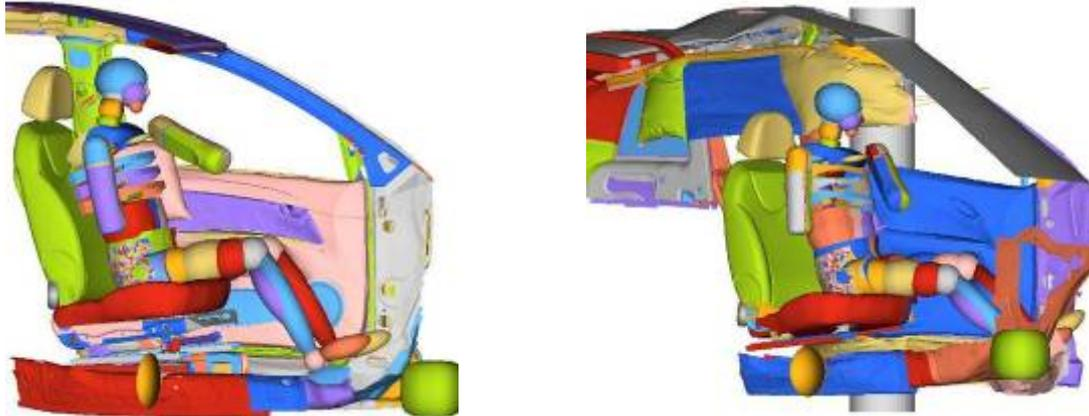
Figure 4 Barrier and pole numerical modeling
