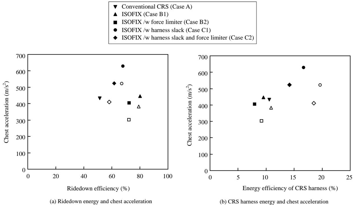
Figure 11 Relation between the energy efficiencies and the chest acceleration. Closed symbols are Hybrid III 3YO FE model and open symbols are child human FE model.
