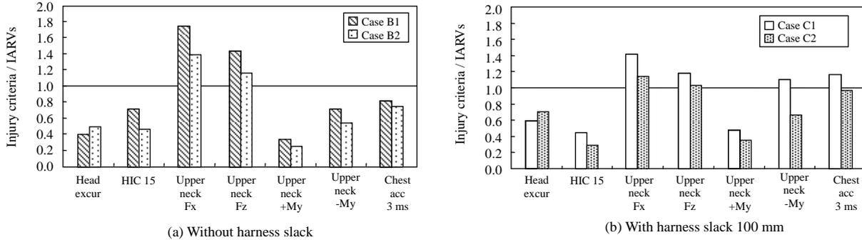
Figure 9 Ratios of injury criteria for Hybrid III 3YO in ISOFIX CRS with (Case B2 and C2) and without (Case B1 and C1) a top-tether force limiter for with and without harness slack
