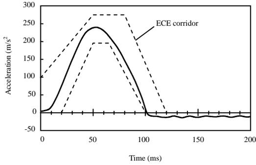
Figure 1 Acceleration pulse in sled test according to ECE R44
