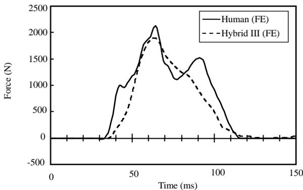
Figure 4 Tension force in the shoulder harness in ISOFIX CRS (Case B1)
