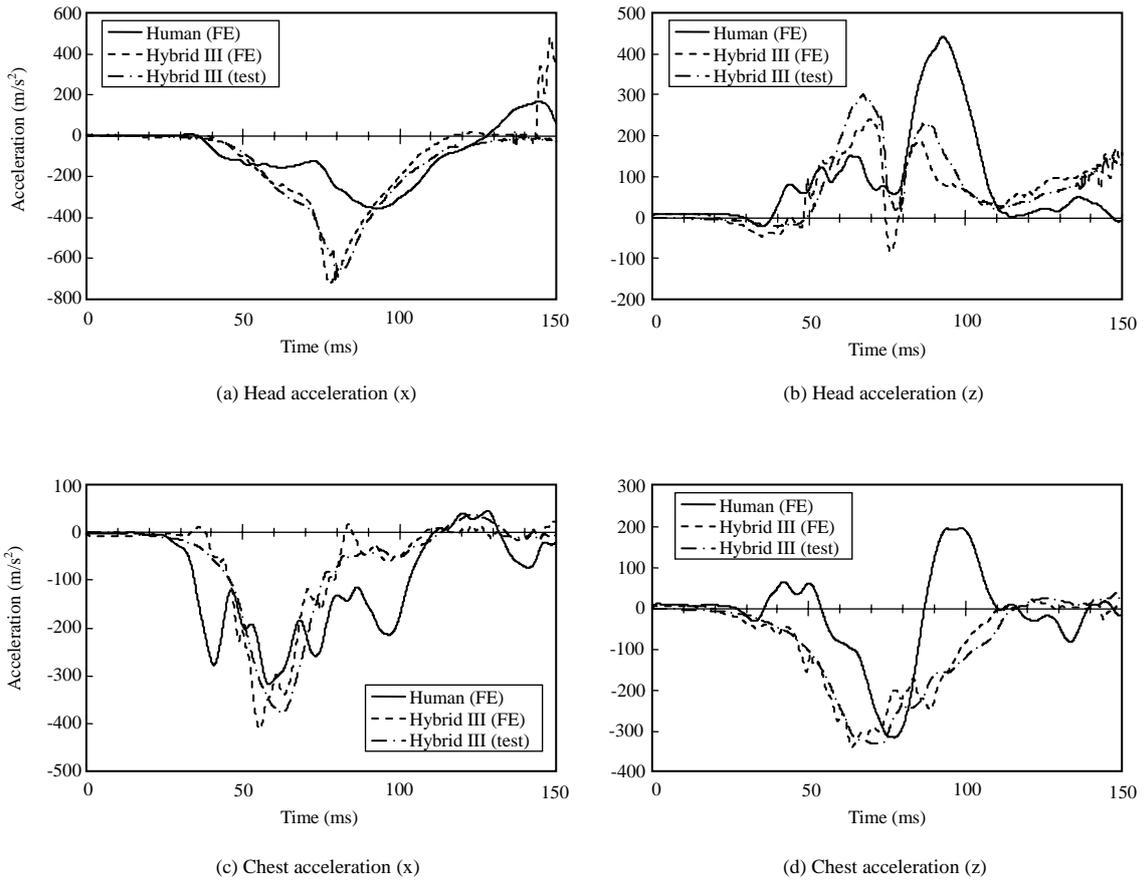
Figure 6 Head and chest acceleration of Hybrid III dummy and human model in ISOFIX CRS (Case B1)
