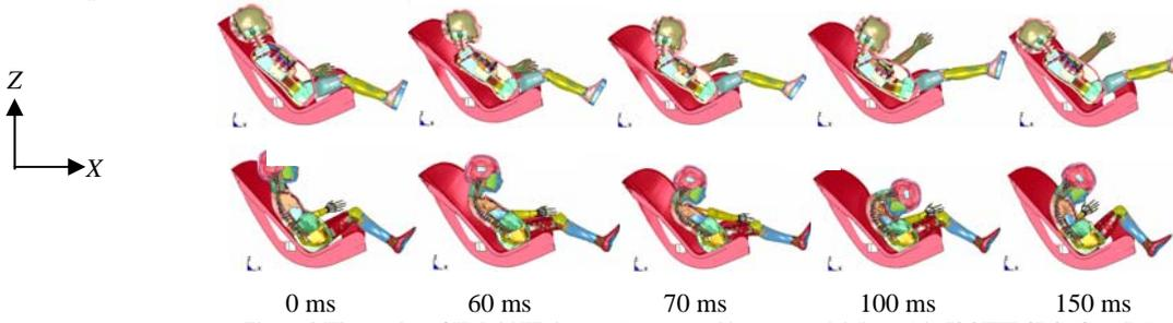
Figure 3 Kinematics of Hybrid III dummy (upper) and human model (lower) in ISOFIX CRS (Case B1)
