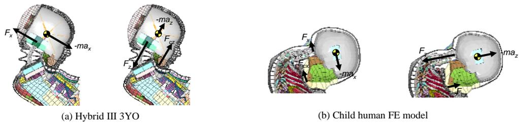
Figure 8 Equilibrium of head forces for Hybrid III dummy model and human model in ISOFIX CRS (Case B1)
