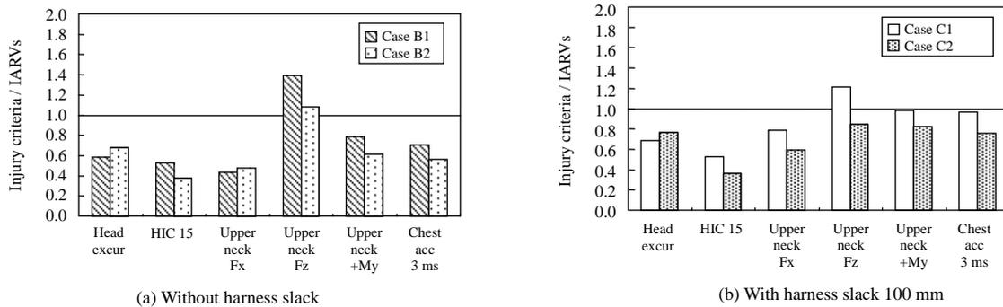
Figure 10 Ratios of injury criteria for child human model in ISOFIX CRS with (Case B2 and C2) and without (Case B1 and C1) a top-tether force limiter for with and without harness slack
