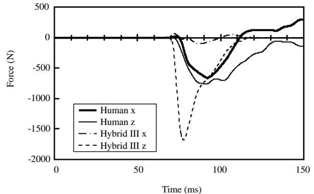
Figure 5 Chin-chest contact force of Hybrid III dummy and human model in ISOFIX CRS with respect to the head coordinate system (Case B1)
