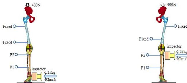
Figure 4. FE simulation of shearing (left) and bending (right) test condition
