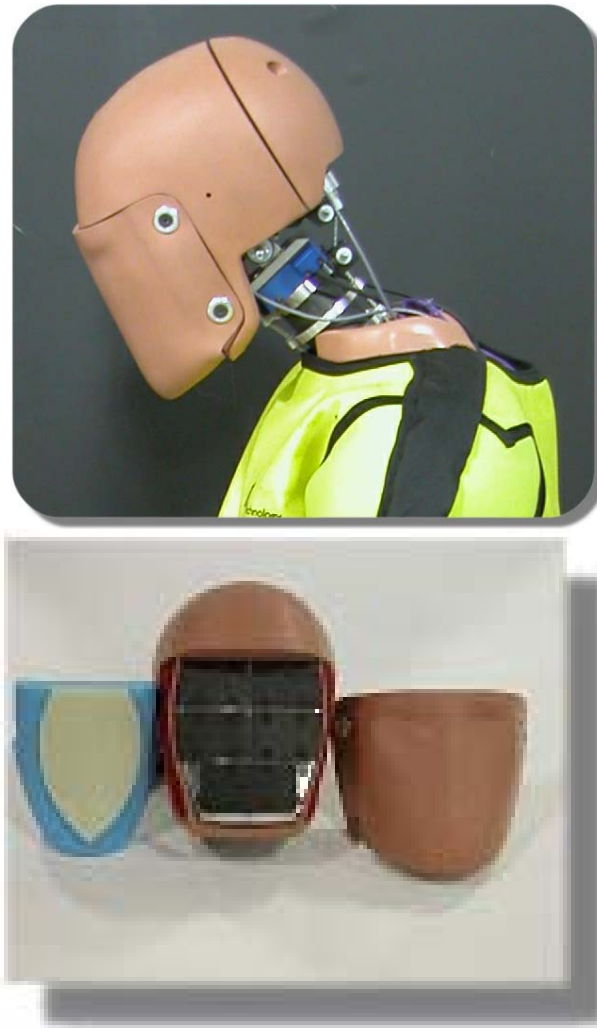
Figure 3 Crash Dummy, Head and Neck (THOR)
