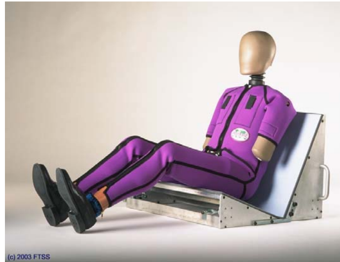
Figure 7 Crash Dummy and Body (WSID)
