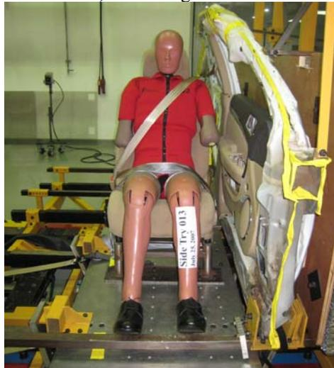
Figure 6 Sled Test Set Up
