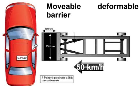
Figure 1 Target Vehicle, struck by Moveable Deformable Barrier.
