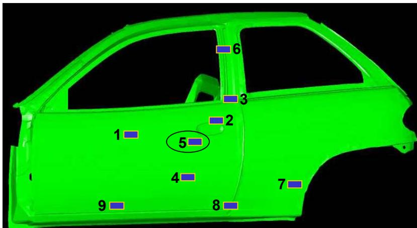
Figure 3 Accelerometer Locations
