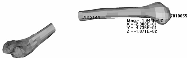
Figure 5 Cortical humerus bone at end of simulation
