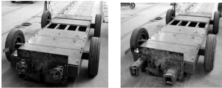
Fig.4 The thickness 1.0mm and 1.5mm square column sled crash tests
