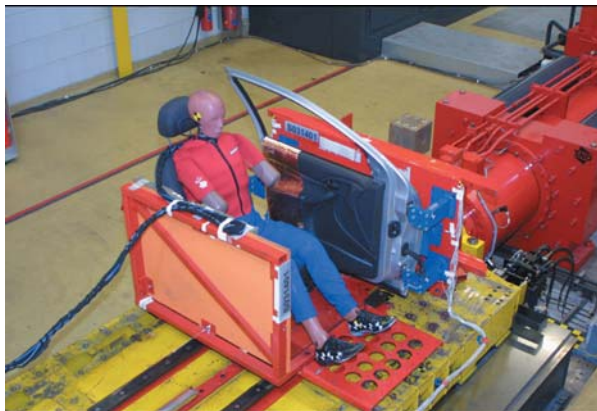
Fig.2 BASIS*. The test set-up is a frame (1) on which the door (2) is mounted. Next to it a seat, with a dummy, is placed on a smaller sled (3), running on linear rails (4). Both the frame and the rails are attached to the ICS sled.
