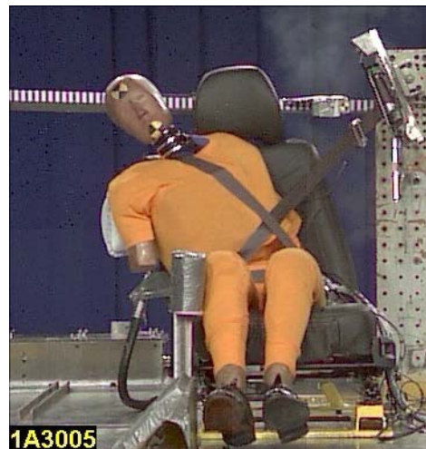
Fig. 4 Cross belt under test [45]
