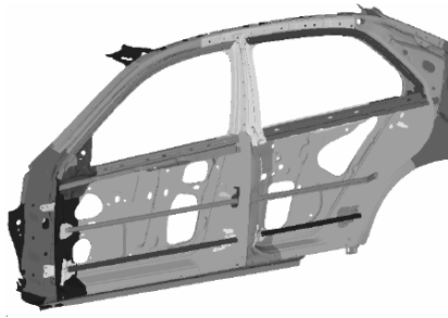
Fig. 1 Side structure of the selected car
