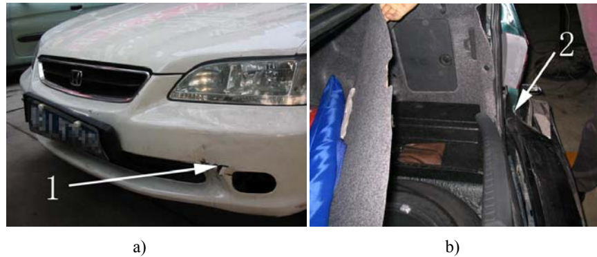
Figure 1 Damages of the accident car.
