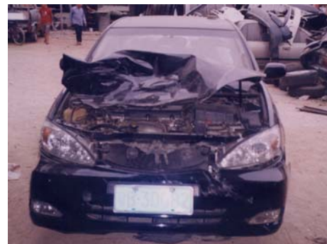
Figure 5 Head damage crossing road after impact (see Figure 3).
