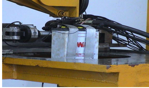
Figure 8 Excide battery fix on the test-bed
