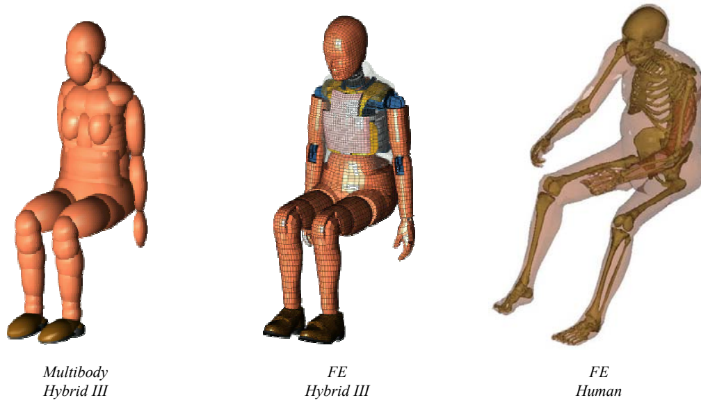
Figure 8: Typical MADYMO dummy & human models (see the Annex for an overview)
