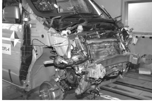
Figure 5. Shear deformation of vehicle in full-width deformable barrier test
