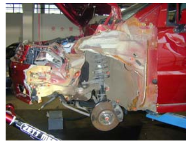
Fig.3 Measure the deformation of auto-body
