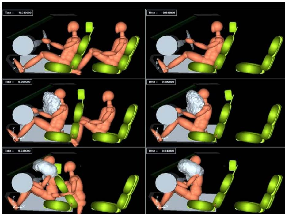
Figure 2: MADYMO<sup>®</sup>-Simulation of occupant kinematics (Dummy Model)
