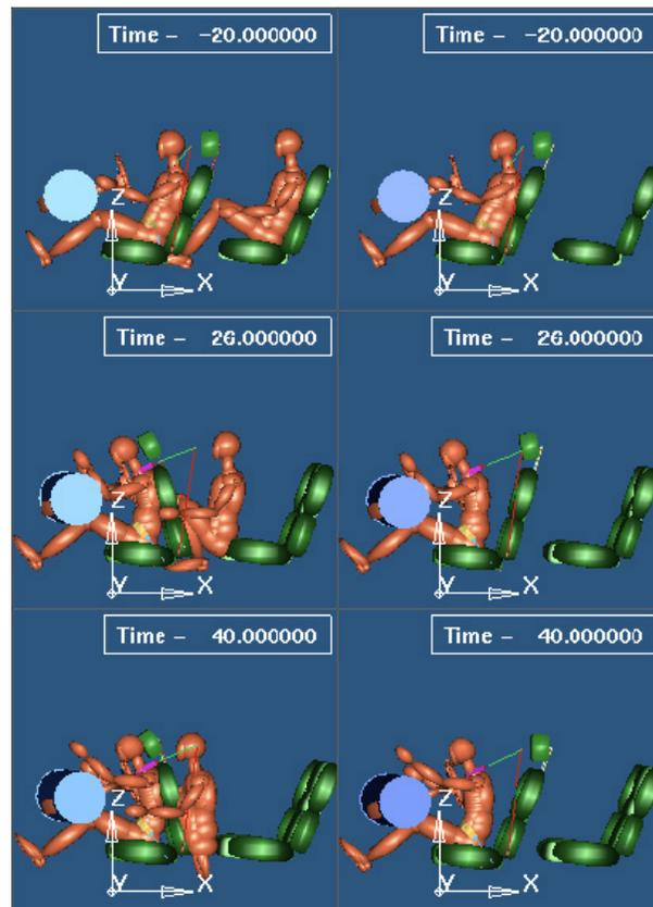
Figure 6: MADYMO®-Simulation of occupant kinematics (Dummy Model)
