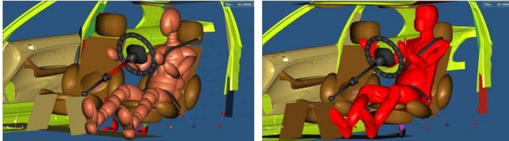
Fig. 9: Dummy and human occupant model in driving position.
