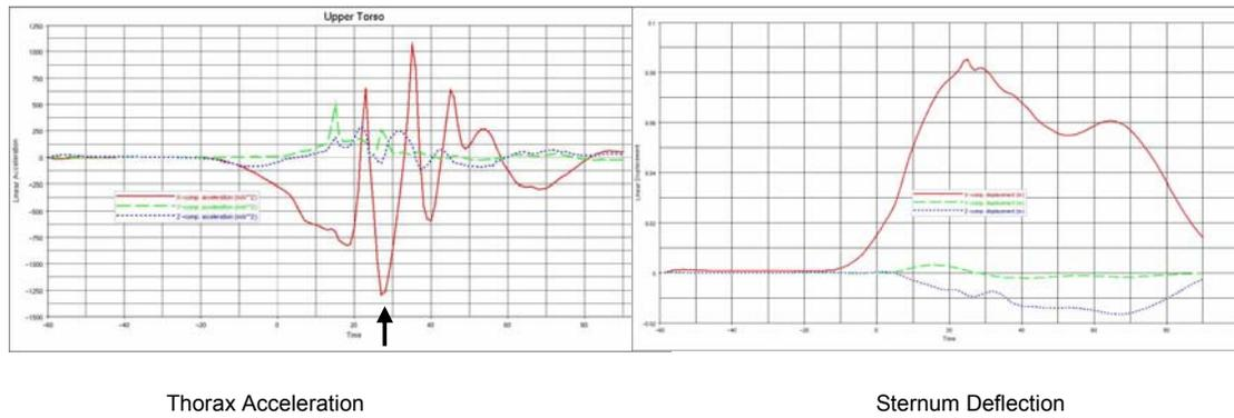
Figure 7: Loading Parameters Thorax (Impact of rear seat passenger)
