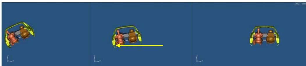
Figure 12: Vehicle kinematics: "sliding into a gravel pit " from right to left
