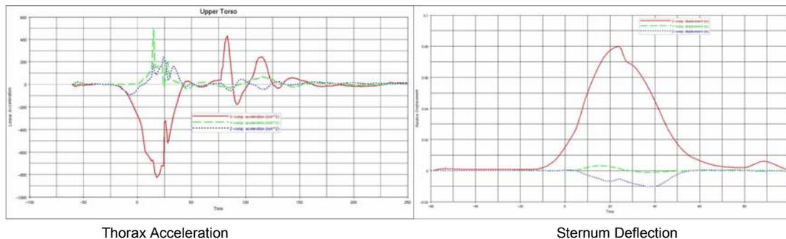
Figure 8: Loading Parameters Thorax (No impact of rear seat passenger)
