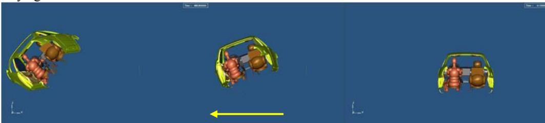
Figure 10: Vehicle kinematics: "sliding against a curb" from right to left
