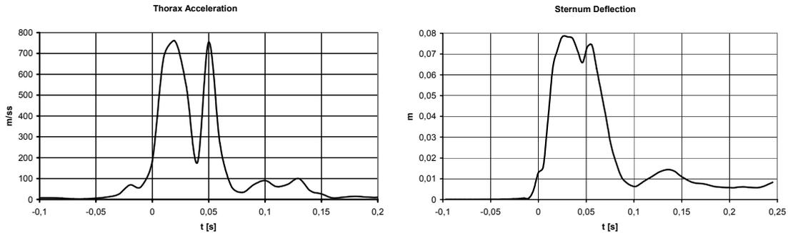
Figure 3: Loading Parameters Thorax (Impact of rear seat passenger)
