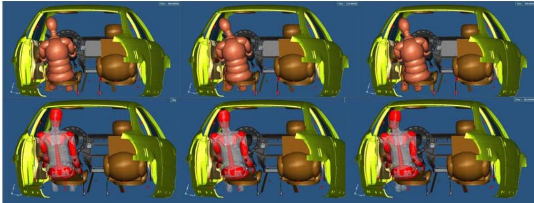
Figure 13: Significant occupant positions (dummy model above human model)
