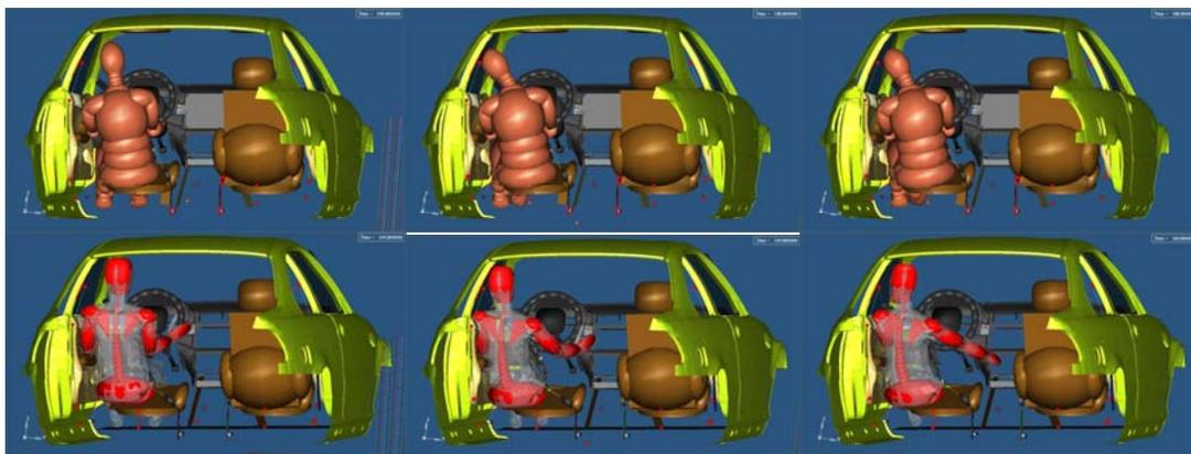
Figure 11: Significant occupant positions (dummy model above human model)
